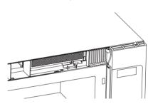
9. Reinstall the vent by sliding the bottom of the vent into place. Push the vent top into position and slide right into place. Replace the two vent mounting screws located on top of the microwave using a #1 Phillips screwdriver.
